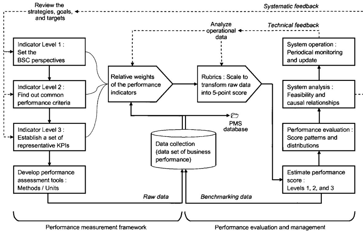
Fig. 1. Implementation model of a PMS for construction companies
